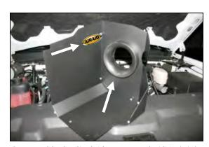
**8.** Assemble the Cool Air Dam panels (CAD) (#2 & #3) using five 6-32 x 5/16" screws (#10), #6 flat washers (#11), and 6-32 keps nuts (#12). Next install the air filter adapter (#5) into the panels as shown with the hole for the Mass Air Flow sensor facing up, using three 1/4 - 20 x 1/2" button head bolts (#14), and 1/4" flat washers (#15). Place the Airaid Decal on the panel as shown.
