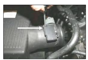
**5.** Remove, and set aside the **MAF** (**Mass Air Flow**) sensor from the factory airbox. This will require a T15 Torx Bit.
