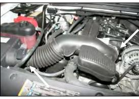
**4.** Loosen two hose clamps on the factory intake tube. One at the throttlebody, and one where it clamps to the factory airbox. Remove the factory intake tube from the vehicle.
