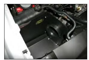
9. Install the Airaid CAD assembly into the vehicle replacing the factory airbox. Secure the CAD using four M6 x 1.25 Hex Bolt (#16), and 1/4" flat washers (#15). Do not over tighten the four bolts
