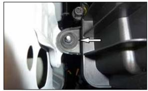
4. Remove the nut that secures the air filter housing into the vehicle and then lift up and remove the air filter housing from the vehicle.
