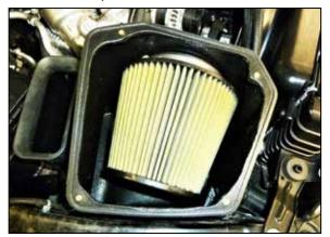
9. Slide the air filter onto the filter adapter and secure with the provided hose clamp.
