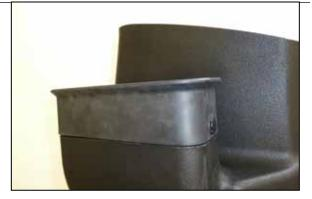
5. Using the provided push pins, install the fresh air intake hood seal onto the K&N air filter housing.
