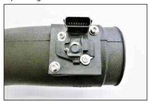
13. Install the mass air sensor assembly into the AIRAID intake tube and secure with the provided hardware. Be sure to install the sensor in the correct direction as shown.
