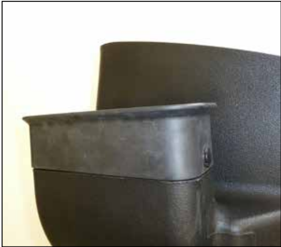
5. Using the provided push pins, install the fresh air intake hood seal onto the K&N air filter housing.
