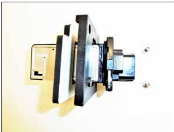
12. Remove the mass air sensor from the factory air filter housing. Assemble the mass air sensor, adapter and gasket as shown. NOTE: 2024 model year vehicles and later have different mass air sensor, the connector lays flat as compared to the sensor pictured.
