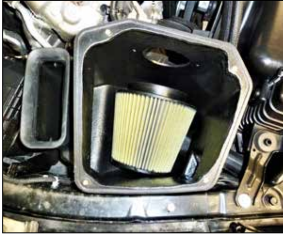
7. Set the air filter into the filter housing.
