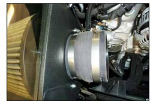
11. Install the provided hump coupler onto the filter adapter and secure with the provided hose clamp.
