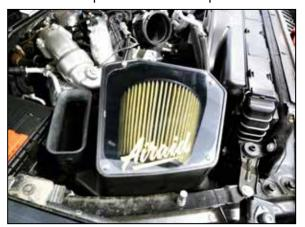
10. Install the lid onto the air filter housing as shown and secure with the provided hardware.
