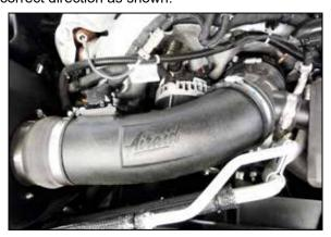
14. Install the intake tube assembly into the coupler at the filter adapter and then into the factory coupler, adjust the tube for best fit and secure with the hose clamps.
