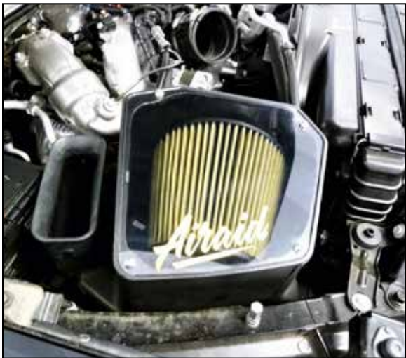
10. Install the lid onto the air filter housing as shown and secure with the provided hardware.
