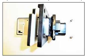
12. Remove the mass air sensor from the factory air filter housing. Assemble the mass air sensor, adapter and gasket as shown.
