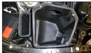
6. Set the AIRAID air filter housing into the vehicle so the studs protrude into the factory mounting grommets.
