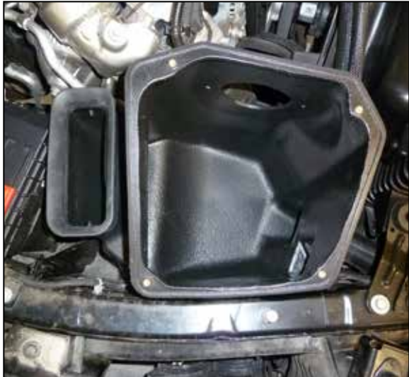
6. Set the AIRAID air filter housing into the vehicle so the studs protrude into the factory mounting grommets.
