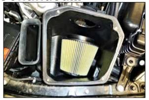
7. Set the air filter into the filter housing.
