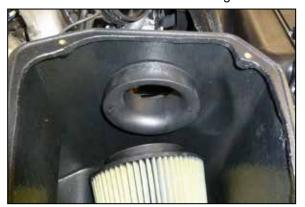
8. Install the filter adapter into the filter housing and secure with the provided hardware.
