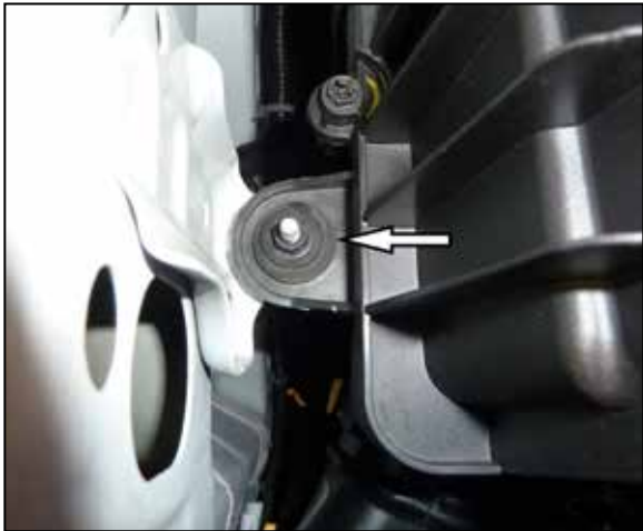
4. Remove the nut that secures the air filter housing into the vehicle and then lift up and remove the air filter housing from the vehicle.
