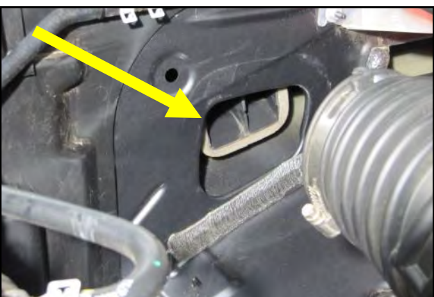
19. On Duramax Powered vehicles, maximum power is achieved by removing the airbox duct in the inner fender.
