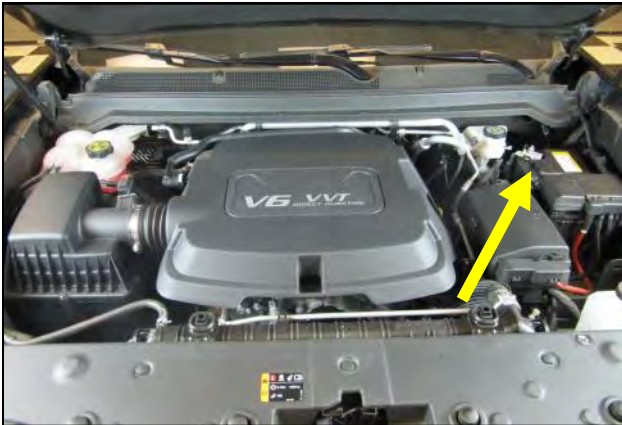
1. Disconnect the negative battery terminal.
