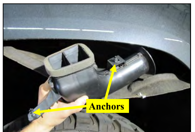
21. Gently pry out the two plastic anchors securing the air duct and remove it. Reinstall the fender liner.
