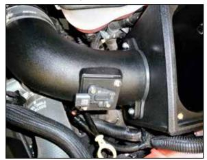
23. Install the intake tube into the coupler and align with the filter housing, then slide the gasket between the tube and housing, insert the filter adapter through the housing and gasket into the intake tube. Align the mounting holes and then secure with the provided hardware.
