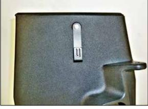
14. Install the wiring harness bracket onto the AIRAID air filter housing using the provided hardware.
