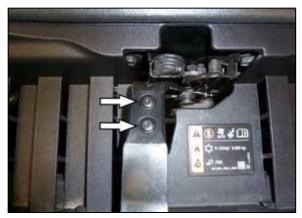
2. Remove the two screws that secure the hood release lever and then remove the lever from the vehicle.
