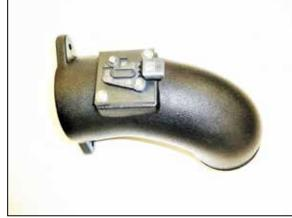
22. Install the mass air sensor into the intake tube and secure with the provided hardware. Note the direction of the mass air sensor when installed should be as in the photo.
