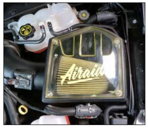
27. Install the AIRAID lid onto the air filter housing and secure with the provided hardware.
