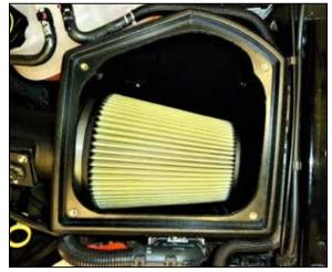
26. Install the AIRAID air filter into the air filter housing and onto the filter adapter, then secure with the provided hose clamp.
