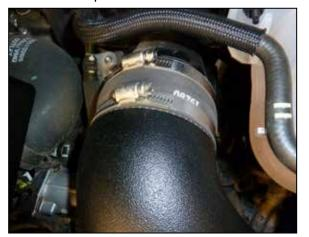
24. Secure the intake tube with the provided hose clamp.
