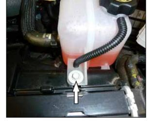
11. Remove the expansion tank mounting bolt shown.
