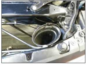
14. Push the factory fresh air intake duct into the AIRAID<sup>®</sup> air filter housing and then reinstall the plastic clip to secure it into position.
