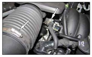
4. Loosen the hose clamps that secure the intake plenum assembly to the throttle body and air filter housing. Disconnect the plenum from the air filter housing and then rotate the plenum assembly counter clockwise to disengage the keyed mount and then remove the plenum from the throttle body.
