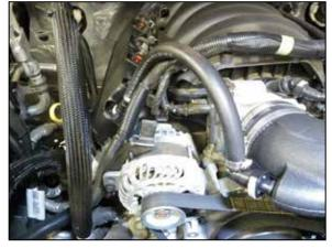
23. Install the crank case vent hose assembly onto the valve cover port and onto the  $90^{\circ}$  fitting on the intake tube.
