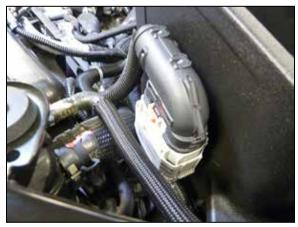
15. Clip the wiring harness onto the bracket installed onto the AIRAID<sup>®</sup> air filter housing.
