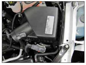
9. Remove the nut that secures the air filter housing assembly to the vehicle. Remove the air filter housing assembly from the vehicle. **NOTE: Go slow and use caution to remove the**
