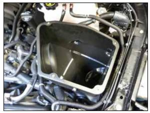
13. Install the AIRAID<sup>®</sup> air filter housing into the vehicle so the mounting grommets engage into the factory mounting holes. Secure the housing with the factory nut removed in step #9.
