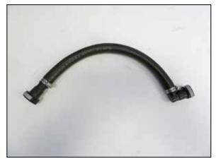
21. Assemble the crank case vent assembly using the provided hose, straight quick disconnect fittings and hose clamps as shown.
