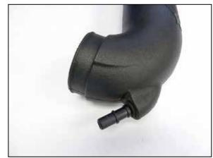
20. Install the grommet and quick disconnect vent
