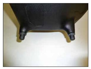
12. Remove the two factory mounting grommets from the factory air filter housing and install them onto the AIRAID<sup>®</sup> air filter housing.
