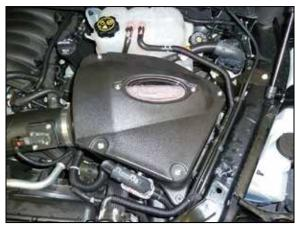
27. Install the AIRAID<sup>®</sup> air filter housing lid onto the air filter housing and secure with the provided hardware.
