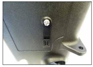
11. Install the provided wiring harness bracket onto the AIRAID<sup>®</sup> air filter housing and secure with the provided hardware.
