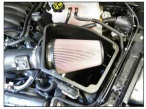
24. Install the AIRAID<sup>®</sup> air filter onto the filter adapter and secure with the provided hose clamp.
