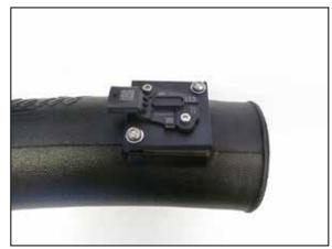
19. Install the mass air sensor assembly into the AIRAID<sup>®</sup> intake tube in the direction shown and secure with the provided hardware.
