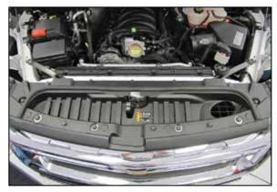
6. Release the ten plastic locking pins holding the upper radiator valence and then remove the valence from the vehicle.
