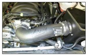
22. Install the AIRAID<sup>®</sup> intake tube into the coupler at the air filter housing and then into the coupler on the throttle body, adjust the tube for best fit and then secure with the provided hose clamps.
