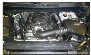
**30. Double check your work!** Make sure there is no foreign material in the intake path. Make sure all clamps, hoses, bolts, and screws are tight. Double check the hood clearance! **Reconnect the negative battery cable!**
