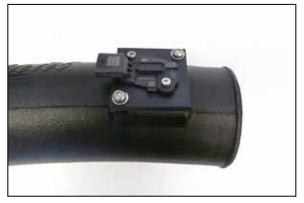
19. Install the mass air sensor assembly into the AIRAID® intake tube in the direction shown and secure with the provided hardware.
