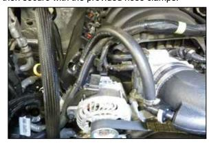
23. Install the crank case vent hose assembly onto the valve cover port and onto the 90° fitting on the intake tube.
