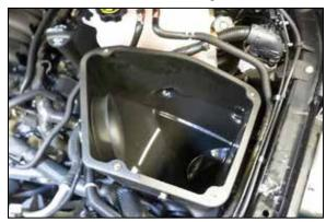
13. Install the AIRAID® air filter housing into the vehicle so the mounting grommets engage into the factory mounting holes. Secure the housing with the factory nut removed in step #9.
