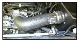
22. Install the AIRAID® intake tube into the coupler at the air filter housing and then into the coupler on the throttle body, adjust the tube for best fit and then secure with the provided hose clamps.
