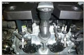
9. Install the engine cover onto the engine and secure the brackets to the factory mounting studs using the factory nuts.
