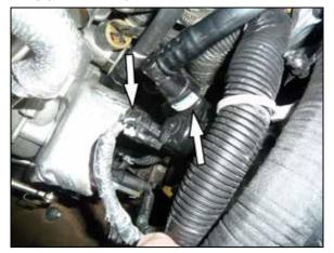
4. Depress the locking tap and then disconnect the CCV pipe from the solenoid attached to the factory intake tube. Disconnect the solenoid electrical connection.
