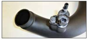
14. Remove the CCV solenoid from the factory intake tube and install it into the K&N intake tube using the factory bolt.
