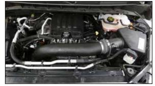
**18. Double check your work!** Make sure there is no foreign material in the intake path. Make sure all clamps, hoses, bolts, and screws are tight. Double check the hood clearance! **Reconnect the negative battery cable!**
