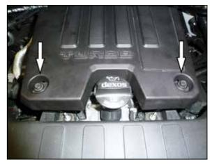
6. Remove the two bolts that secure the engine cover to the engine and then remove the cover from the vehicle. These bolts will be reused in a later step.
