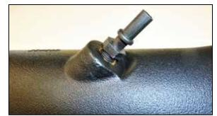
13. Install the provided quick connect fitting into the K&N intake tube.
