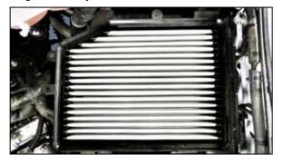
10. Remove the upper air filter housing and remove the factory air filter.
