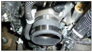
12. Install the provided straight coupler onto the turbo inlet and secure with the provided hose clamp.
