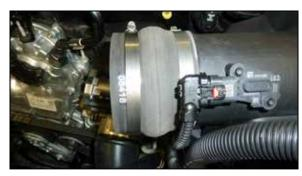
11. Install the AIRAID air filter and then reinstall the upper housing and secure with the factory screws. Install the provided hump coupler onto the air filter housing and secure with the provided hose clamp.
