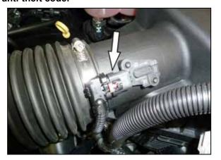
2. Disconnect the mass air sensor electrical connection and loosen the hose clamp that secures the factory intake tube to the air filter housing.
