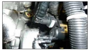
17. Connect the CCV tube to the solenoid and connect the electrical connection.
