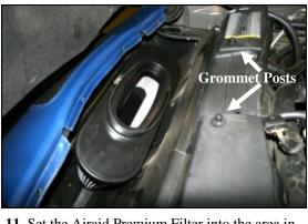
**11.** Set the Airaid Premium Filter into the area in front of the radiator. It will be mounted in step # 15
