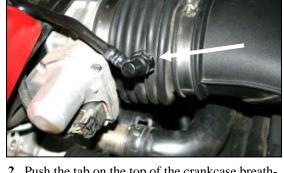
**2.** Push the tab on the top of the crankcase breather connector, and disconnect the breather hose from the factory intake tube breather fitting.
