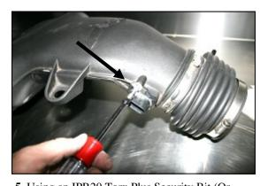
Equivalent) remove the two factory screws that hold the **MAF** sensor into the factory intake tube. Remove the **MAF** sensor for reinstallation in step #9.
