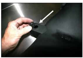
**8.** Install the two factory grommets that were removed in step #4, into the Airaid Intake Tube as
