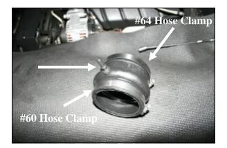
**4.** Reinstall the barbed fitting removed in step #3 into the Airaid hump hose (#3) as shown. Install one #64 hose clamp (#14) onto the back of the hump hose, and one #60 hose clamp on the front.
