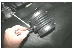
**3.** Remove the barbed fitting from the factory coupler. It will be reused in step #4.
