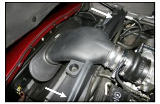
11. Install the supplied weather strips (#7) on top of the air dams as shown. Pull the Airaid Premium Filter up and secure it onto the Airaid intake tube with the supplied hose clamp.
