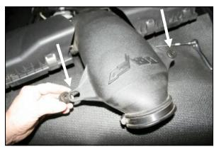
**5.** Remove the two factory grommets from the factory intake tube. They will be reused in step #6.
