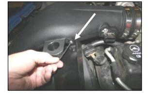
14. Tighten all four button head bolts that secure the air dams to the intake tube, and the radiator shroud.
