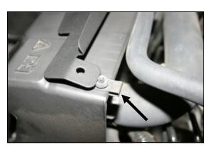
13. Slide one clip nut (#10) over the outside end of the plastic radiator cover and align it with the hole in the air dam. Install one rubber washer (#11) over the threads of the clip nut, and then align the air dam hole over the washer. Add one more rubber washer, one #8 flat washer (#9), and one M4 Pan Head Screw (#8) to secure the air dam. Repeat this step on the passenger side. Refer to the line drawing on page one.
