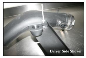
8. Attach the two air dams (#5 driver side & #4 passenger side) onto the Airaid Intake Tube using one 8-32x1/4" button head bolt (#8) and #8 flat washer (#9) on each side. Leave the bolts slightly loose for now to allow for adjustment.
