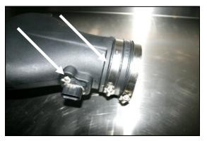
7. Reinstall the Mass Air Flow sensor removed in step #4, into the Airaid Intake Tube using two 8-32x3/8" button head bolts (#7). **Do Not Use The Factory Screws!**
