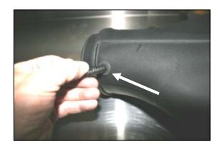
screws that hold the MAF sensor into the factory intake tube. Remove the MAF sensor for reinstallation in step #7.
