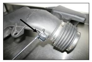
4. Using a #20 Torx Bit, remove the two factory
