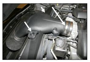
12. Install the Airaid Intake Tube assembly onto the throttle body first, and then align the grommets over the factory grommet posts on top of the radiator shroud. Push down on the grommets to seat them on the posts. (*Hint: Use a 1/2" deep* socket to help seat the grommets onto the posts.) Now tighten the hose clamp on the throttle body.
