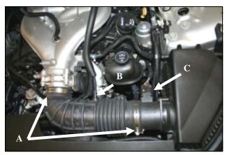
**2. A)** Loosen the hose clamps on the factory intake tube.
