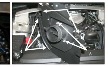
**9. A)** Transfer the Mass Air Flow Sensor from the factory airbox to the Adapter Panel and secure using two 1/4-20 button Head Screws (#15) and Serrated Nuts (#17). Note: The factory airbox seal on the Mass Air Flow Meter is not to be used in this kit. **B)** Attach the Weather Strip (# 11) to the curved edge of the MAF Panel. **C)** Insert the 5/8" hose anchors (#28) into the two horizontal tab holes on the MAF panel.
