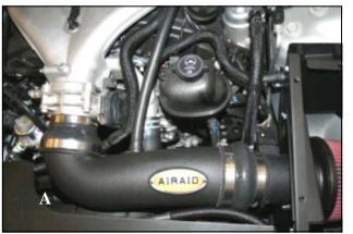
**13.A)** Install the Airaid Intake Tube assembly onto the Mass Air Flow Sensor first, and then onto the throt-tle body. Adjust for fit, and tighten the hose clamps. **B**) Replace the factory breather line on the valve cover with the 26" Airaid Breather Hose(#11). Secure the breather hose to the intake tube nipple using the black Speed Clamp (#29).Apply the Airaid Bubble Decal onto the Intake Tube as shown.
