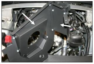
**6.** Install the Adapter Panel (#5) to the MAF Panel (#3) as shown using four 6-32 screws (#12), 6-32 Kep nuts, and #6 flat washers (#14). Attach the Rear Panel (#4) to
