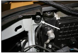
**4.** Use caution not to loose the factory core support grommet while removing the airbox assembly. It will be used in step 11.
