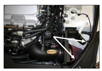
12. Install the Airaid Intake Tube (#2) assembly onto the filter Adapter first, and then onto the throttlebody. Adjust for fit, and tighten all 3 hose clamps. Next reconnect the MAF sensor and Breather line. Slide the Edge Clip Cable Ties (#30) about 6" apart along the fender pinch weld and return the coolant line to it's original location. Secure the coolant line using the cable ties and trim off
