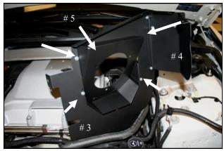
**5.** Install the Adapter Panel (#5) to the MAF Panel (#3) as shown using four 6-32 screws (#12), 6-32 Kep nuts, and #6 flat washers (#14). Attach the Rear panel (#4) to the MAF panel using two 6-32 screws.
