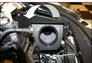
11. A) Locate and remove the Factory Ground strap bolt in the chassis. B) Lower the Airaid Performance Airbox assembly into the engine cavity. Insert the Well Nut into the Factory core support grommet and rotate the assembly rearward until the bracket rests on the shock tower and the MAF panel's lower tab hole is lined up with the Chassis bolt hole. Secure the assembly by reusing the factory 6mm Chassis Bolt.
