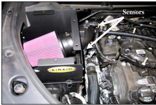
**11.** Install the Airaid Premium Filter (#1) to the Intake Tube. Reconnect the **M**ass **Air** Flow and **MAP** sensors.
