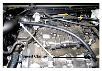
**10.** Attach the 1/2" Breather Hose to the Intake Tube nipple and the factory valve cover fitting. Secure using the Speed Clamps (#17).
