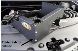
**5.** Join the two Airaid panels together with the folded tabs on the **outside**, using the four 6-32 screws (#15), #6 Flat washers (#14), and #6 Keps Nuts (#13). Apply the Airaid Foil Decal onto the Panel as shown.
