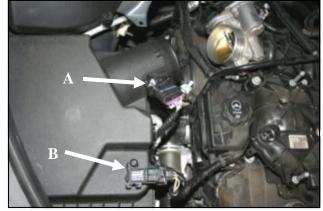
**3.** Disconnect the Mass Air Flow, or MAF sensor (A) and the MAP sensor (B) from the factory airbox lid.
