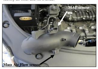
7. Transfer the air sensors from the factory airbox lid into the Airaid Intake Tube(#2) as shown. **Do Not Use**The Factory Hardware. Secure the Mass Air Flow sensor using the two #8-32 screws (#16), and the MAP sensor using the 1/4-20x 3/4 hex head bolt (#9) and 1/4" Flat Washer (#12).
