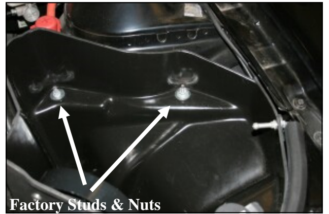
12. Install the Airaid Cold Air Box into the vehicle locating the factory grommets over the factory studs. Reinstall the factory nuts from step #3 onto the studs. Reinstall the factory ground lug thru the Airbox wall.
