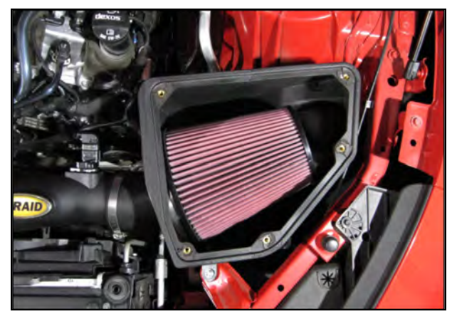
24. Install the Air Filter onto the filter adapter, inside the Airbox.
