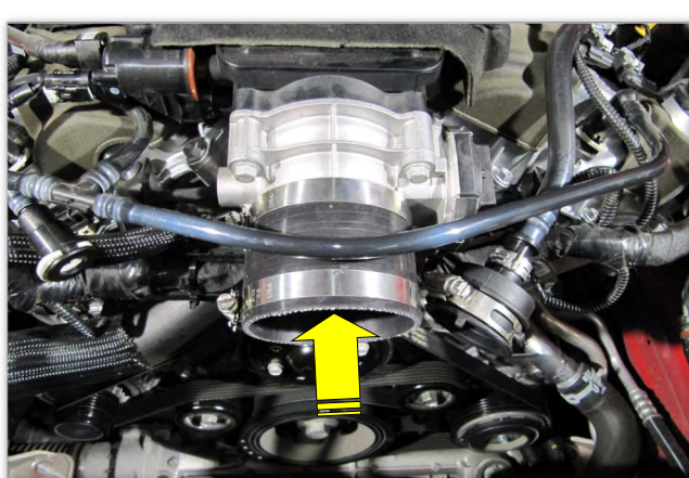
20. Slide the Coupler and #48 Clamps onto the throttle body as shown.
