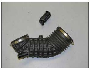
15. Cut the clamp that secures the PCV chamber into the factory intake tube and then remove the chamber from the tube.
