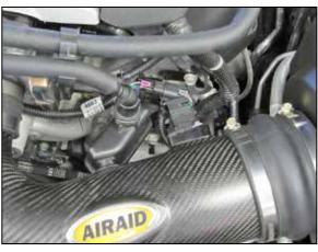
19. Connect the crank case vent hose to the PCV vent chamber and connect the mass air sensor electrical connection.
