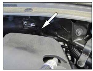
8. At the firewall, Remove the 6mm flange nut that secures the sound tube to the firewall. Turn the tube  $\frac{1}{4}$  turn clockwise and the remove the tube from the vehicle.
