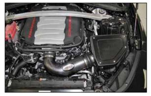
23. Double check your work! Make sure there is no foreign material in the intake path. Make sure all clamps, hoses, bolts, and screws are tight. Double check the hood clearance! Reconnect the negative battery cable!
