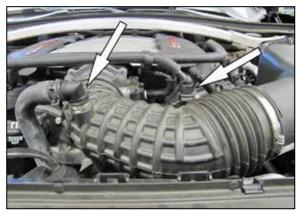
2. Release the spring clamp securing the resonator tube to the 90 deg. Fitting and then disconnect the tube. Depress the locking tab and then disconnect the crank case vent hose.
