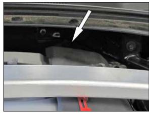
9. Install the provided plug into the sound tube hole.
