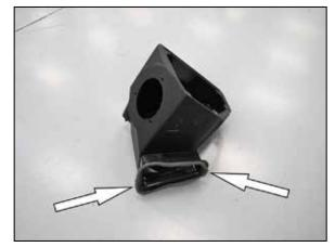
10. Remove the air box inlet from the factory air filter housing and install it onto the AIRAID air filter housing.
