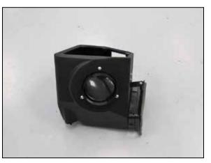
12. Install the radius filter adapter into the AIRAID filter housing and secure with the provided hardware.
