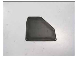
21. Install the provided gasket onto the air filter housing lid.
