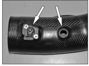
13. Remove the mass air sensor from the factory air filter housing and install it into the AIRAID intake tube with the provided hardware. Install the provided crank case grommet into the AIRAID intake tube as shown.
