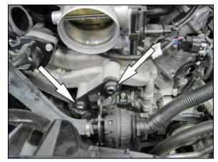
6. Using a T50 TORX, remove the two bolts securing the sound resonator to the front of the engine.
