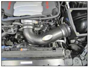
18. Install the coupler houses and hose clamps onto the AIRAID intake tube but do not tighten the clamps. Install the intake tube assembly onto the filter adapter and throttle body. Adjust the assembly for best fit and then secure all the hose clamps.
