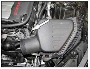
4. Disconnect Mass air flow sensor electrical connection and then lift and remove the complete air filter housing from the vehicle.
