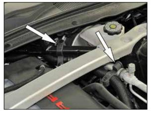
7. Locate and disconnect the sound tube retainers on the strut tower brace and A/C line.
