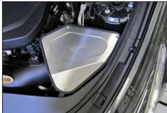
13. Install the provided gasket onto the air box lid, then install the lid onto the air box and secure with the provided hardware.
