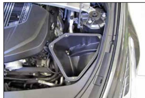
5. Install the AIRAID® air filter housing into the vehicle so the mounting studs engage the factory mounting grooves.
