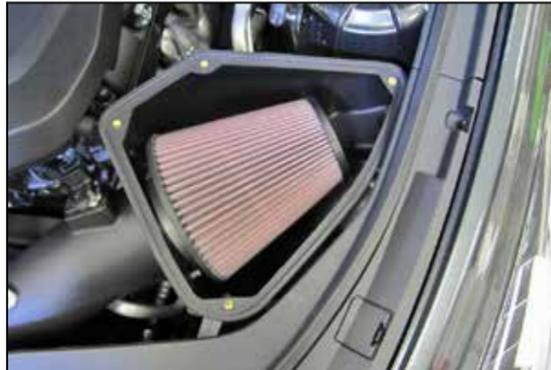
11. Install the AIRAID® air filter onto the intake tube and secure with the provided hose clamp.
