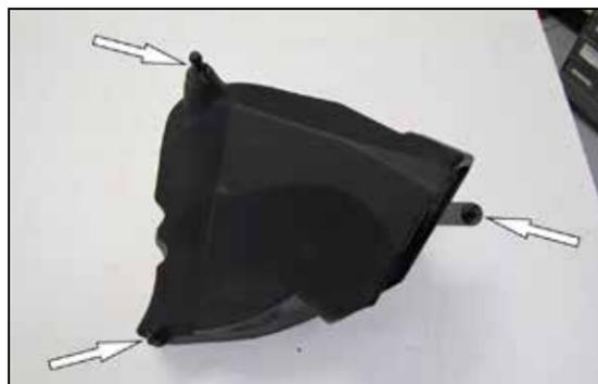
4. Install the provided mounting bracket through the cutout line in the AIRAID® air box and then secure with the provided hardware. Install the provided mounting studs onto the bracket and onto the air filter housing as shown.
