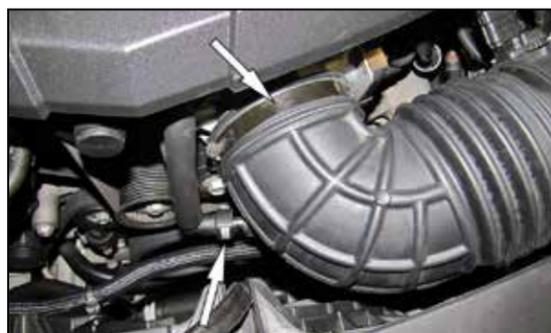
3. Disconnect the crank case vent line and loosen the hose clamp that secures the intake tube to the throttle body. Remove the complete intake system from the vehicle.
