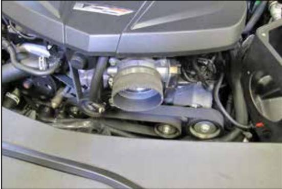
8. Install the provided coupler hose (08761) onto the throttle body and secure with the provided hose clamp.
