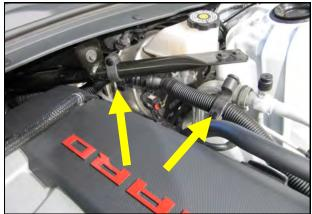
**5.** Separate the resonator tube from the airbox lid. Follow the tube up to the master cylinder area and disconnect the tube retainers on the strut tower brace and the A/C line.
