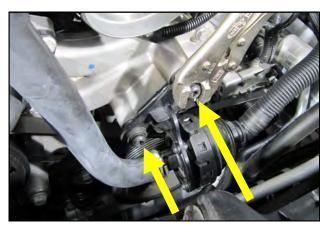
**4.** Remove the two bolts in the resonator diaphragm bracket using a T-50 Torx bit or with a pair of locking pliers as shown. The resonator, bolts and bracket will not be used with the Airaid.
