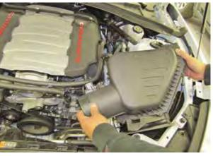
11. Detach and lift the airbox lid and replace the air filter with the provided AIRAID air filter.
