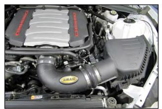
**15.** Slowly lower the hood to test clearances. Make sure all clamps, hoses, bolts, and screws are tight. Double check the hood clearance. Reconnect the negative battery terminal and re install the access panel.
