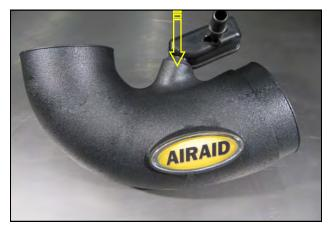
**10.** Transfer the PCV fitting into the Intake tube and apply the Airaid Decal as shown.
