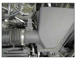
3. Slide the locking tab back and then disconnect the mass air sensor electrical connection.
