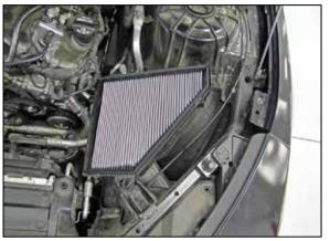
9. Remove the air filter housing lid and replace the stock air filter with the provided AIRAID filter, reinstall the lid and secure with the factory hardware.
