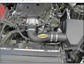
13. Install the intake tube into the coupler at the air filter housing and then into the coupler at the throttle body, adjust the tube for best fit and then secure with the provided hose clamps. Connect the EVAP and crank case vent lines.
