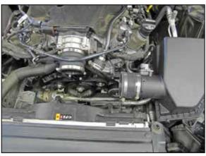
12. Install the coupling hoses onto the air filter housing and throttle body as shown.
