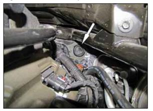
8. Install the provided plug into the hole for the sound tube in the firewall.
