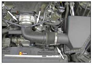
4. Loosen the hose clamp that secures the EVAP line and unclip the crank case vent to the intake tube and disconnect them. Loosen the two hose clamps that secure the intake tube to the air filter housing and throttle body. Disconnect the tube from the air filter housing and throttle body.
