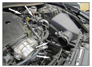
6. Release the four sound drum tube mounts.
