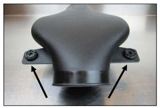
**3.** Transfer the factory intake tube mounting grommets into the Tube Brackets as shown.
