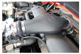
6. Check the alignment of all the intake components and adjust if necessary. Begin tightening the clamps from the front of the intake and move back towards the throttle body. Reconnect the battery.
