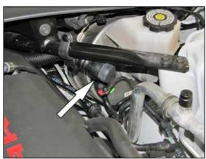
11. Install the cap assembly into the remaining sound tube.
