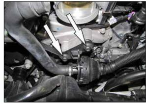
6. Remove the two bolts securing the sound drum to the front of the engine.
