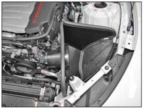
20. Install the AIRAID® heat shield assembly onto the air filter housing mounting grommets.
