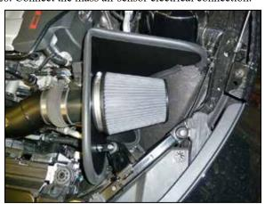
27. Install the AIRAID® air filter and secure with the provided hose clamp.
