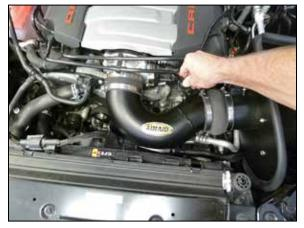
25. Connect the crank case vent hose to the quick disconnect fitting installed into the AIRAID® intake tube.
