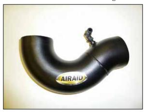
23. Install the provided  $90^{\circ}$  fitting into the AIRAID® intake tube as shown.
