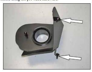
16. Install the remaining two mounting studs onto the heat shield using the provided hardware.
