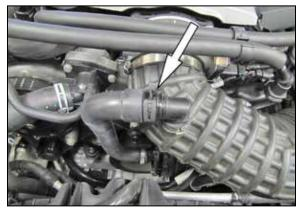
4. Release the spring clamp securing the sound tube to the fitting in the intake tube and then disconnect the sound tube.
