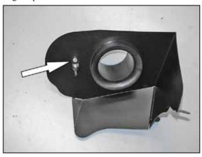
15. Install the mounting bracket assembly onto the heat shield using the provided hardware.
