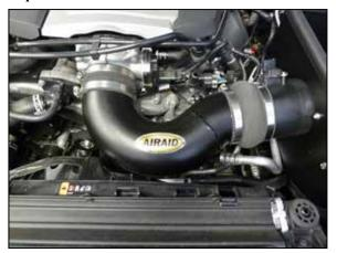
24. Install the AIRAID® intake tube into the hump coupler and then into the coupler at the throttle body, adjust the tube for best fit and then secure with the provided hose clamps.
