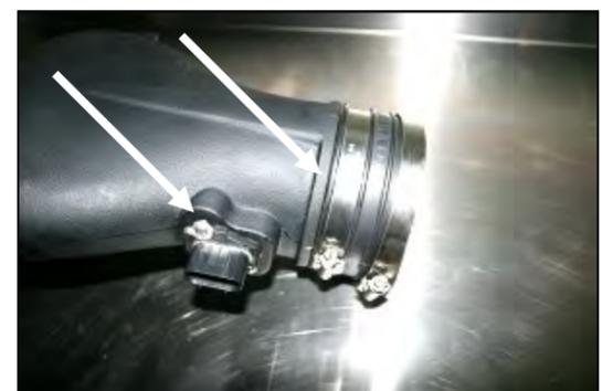
9. Reinstall the Mass Air Flow sensor removed in step #5, into the Airaid Intake Tube using two 8-32x3/8" button head bolts (#7).
