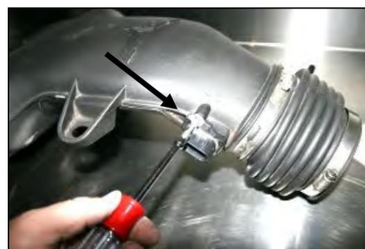
5. Using an IPR20 Torx Plus Security Bit (Or Equivalent) remove the two factory screws that hold the MAF sensor into the factory intake tube. Remove the MAF sensor for reinstallation in step #9.
