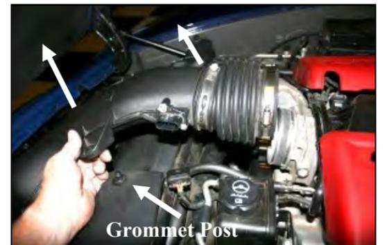
3. Lift up on the factory intake tube assembly to disengage the grommets from the two grommet posts and throttle body. Remove the assembly from the vehicle.
