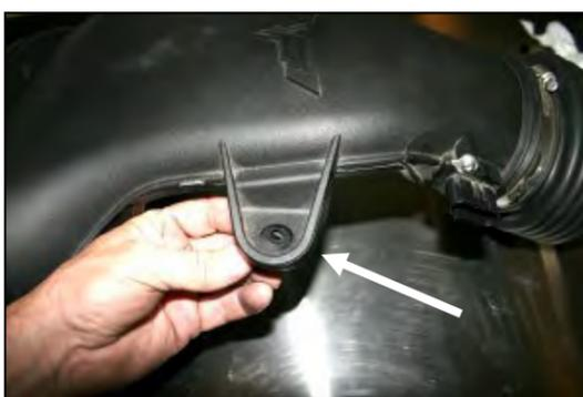
4. Remove the two factory grommets from the factory intake tube and set them aside for reuse in step #8.
