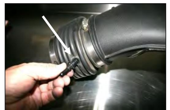
6. Remove the factory breather fitting from the factory intake tube and save for reinstallation in step #7.
