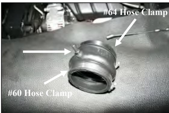
4. Reinstall the barbed fitting removed in step #3 into the Airaid hump hose (#3) as shown. Install one #64 hose clamp (#14) onto the back of the hump hose, and one #60 hose clamp on the front.
