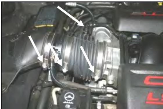
1. **Disconnect negative battery cable.** Push the tab on the factory breather hose and disconnect it from the fitting in the factory coupler. Loosen the three hose clamps on the factory intake tube.
