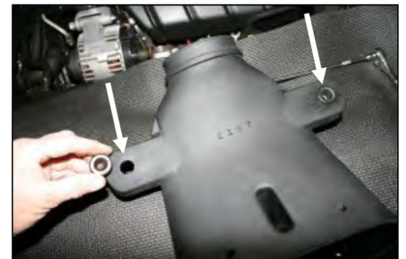
6. Install the factory grommets removed in step #5 into the Airaid intake tube (#2).
