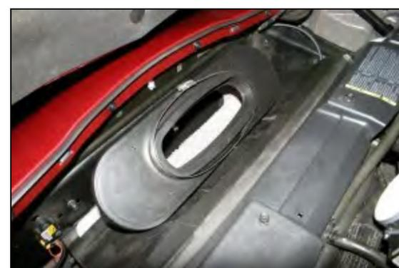
8. Install the Airaid Premium Filter into the area in front of the radiator. It will be attached to the Airaid intake tube in step #11.
