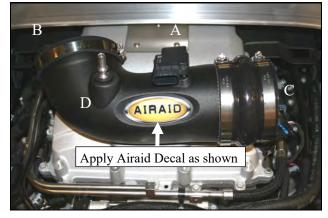
9. A) Transfer the Mass Air Flow sensor from the Factory airbox assembly into the Airaid Intake Tube(#2). Secure to the tube by using the 8-32 screws (#15) and #8 lock washers (#16). B) Install the GM Coupler (#9) on to throttle body side of the intake tube. C) Install the Hump Hose (#10) on the filter side of the intake tube as shown. D) Insert the Grommet (#24) into the hole in the Airaid Intake Tube and then follow by inserting the barbed end of the PCV Fitting (#25) into the Grommet.
