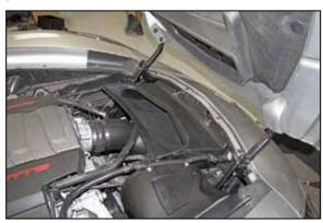
26. Reinstall the radiator heat extractor duct and secure with the factory hardware.
