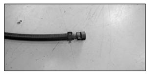
18. Install the provided quick disconnect fitting into one of the provided coolant hoses and secure with the provided spring clamp.
