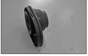
11. Install the outer air filter housing onto the AIRAID® mass air housing and secure with the provided hardware.
