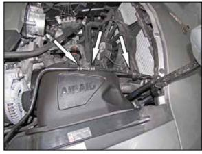
17. Be sure the vehicle is completely cool before beginning this step. Be sure to capture any coolant that leaks from the lines. Using a razor or sharp instrument, cut the nylon coolant lines in the three locations shown. Use multiple shallow cuts so as not to cut too deep and cause damage to the underlying fittings. Remove the nylon coolant lines from the check valve and tee fitting and expansion tank. The check valve should still be attached to the line attached to the radiator.
