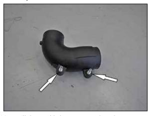
14. Install the provided grommets and crank case vent fittings into the AIRAID® intake tube as shown.
