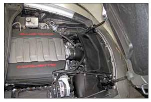
**27. Double check your work!** Make sure there is no foreign material in the intake path. Make sure all clamps, hoses, bolts, and screws are tight.
