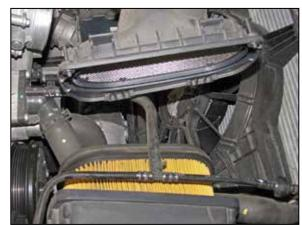
6. Unhook the coolant lines from the air filter housing, then loosen the two screws that secure the mass air portion of the air filter housing and remove it from the vehicle along with the factory air filter.
