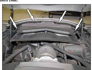
2. Remove the four screws that secure the radiator heat extractor duct to the radiator and then remove the duct from the vehicle.
