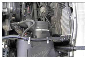
22. Install the provided straight coupler onto the AIRAID® mass air sensor and secure with the provided hose clamp.
