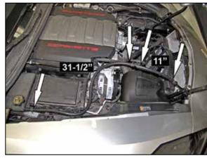
19. Trim the hose with the quick disconnect fitting to 31-1/2" long and trim the remaining hose to 11" long. Install the 31-1/2" long hose from the expansion tank to the tee fitting. Secure the hose with the provided spring clamp, route the hose as shown and secure with the provided tie wraps. Install the 11" hose onto the check valve and tee fitting and secure with the provided spring clamps.
