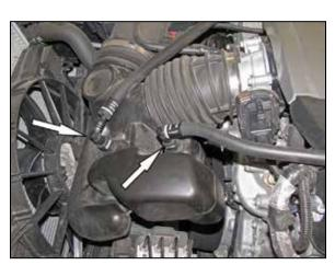
3. Depress the grey locking tabs and then disconnect the crank case vent lines from the factory intake tubes.
