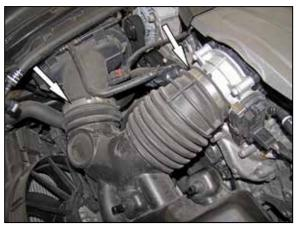
4. Loosen the two hose clamps that secure the factory intake tube to the throttle body and air filter housing and then remove the tube from the vehicle.
