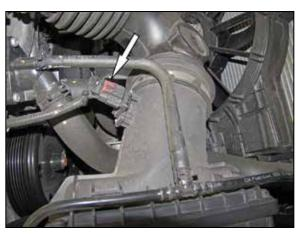
5. Slide the red tab back and then depress the mass air sensor locking tab and disconnect the mass air sensor electrical connection.
