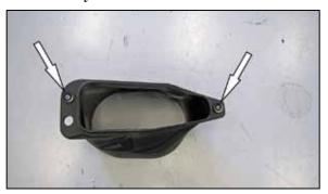
8. Insert the mounting grommets with sleeves into the AIRAID® air filter housing at the two locations shown. NOTE: The rubber grommets will be on both sides of the part with the sleeve passing through them.
