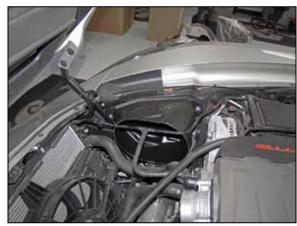
16. Install the AIRAID® air filter housing into the inner fender so that the mounting grommet engages with the mounting stud. Secure the housing with the provided hardware.
