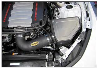
**27.** Slowly lower the hood to test clearances. Make sure all clamps, hoses, bolts, and screws are tight. Double check the hood clearance. Reconnect the negative battery terminal and re install the access panel.
