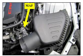
**4.** Disconnect the air flow meter, or MAF, in the air box lid and remove the entire airbox assembly from the vehicle
