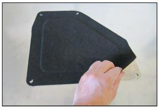
**24.** Prepare the Airbox Lid for Gasket installation by cleaning the mounting surface using a Prep Solvent or equivalent. Remove the adhesive backing from the Gasket and carefully apply it as shown with the screw holes aligned.
