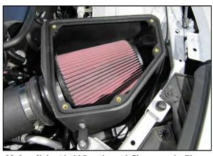
**23.** Install the Airaid Premium Airfilter on to the Fitter Adapter in the Airbox.
