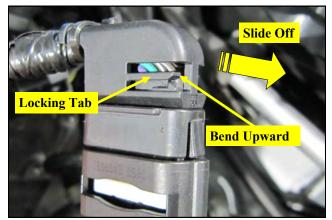
**18.** The connector for the MAF sensor has a 90 degree wire guide on it. Cut the zip tie on the guide. Locate the locking tabs on both sides of the guide and bend the tabs upward to slide the guide off of the connector. This will not be used with the Airaid Intake.
