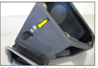
**11.** Slide the Airbox Bracket into the slot above the air inlet, from inside the box, and secure it using two sets of 1/4-20 Button Head Screws and Flat Washers.
