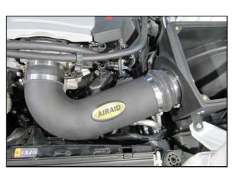
22. Align the Intake Tube and tighten all four Clamps.
