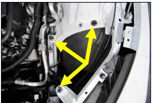
**5.** Ensure that all 3 airbox mounting grommets remain in the vehicle
