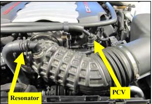
2. Compress the spring clamp on the resonator tube and separate the tube from the 90 deg. fitting in the intake tube. Depress the grey locking tab in the PCV fitting and disconnect the PCV line from the intake.
