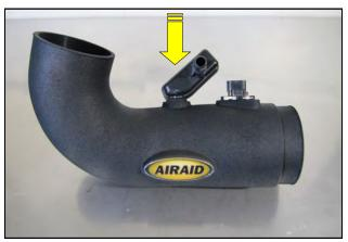
**16.** Transfer the PCV fitting into the Grommet in the Airaid Intake Tube. Apply the Airaid Badge to the Intake Tube as shown.
