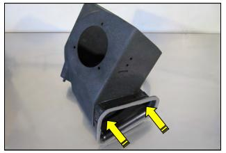
**10.** Transfer the factory air box inlet onto the Airaid air box as shown.
