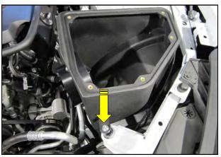
**17.** Place the Airaid Airbox assembly into the engine compartment as shown, with the mounting posts only fully seated in all three grommets.
