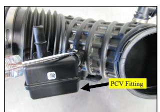
**15.** Using a small flat tip screwdriver, uncrimp the clamp securing the PCV fitting to the intake tube.
