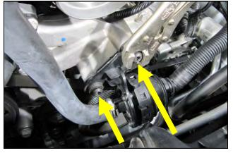
**6.** Remove the two bolts in the resonator diaphragm bracket using a T-50 Torx bit or with a pair of locking pliers as shown. The resonator, bolts and bracket will not be used with the Airaid.
