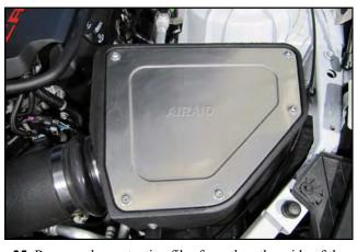
**25.** Remove the protective film from the other side of the Lid and mount it to the Airbox using 5 sets of 1/4-20 Button Heads and Flat Washers.
