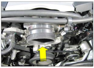
${\bf 20.}$  Slide the Coupler and #60 Clamps onto the throttle body as shown.
