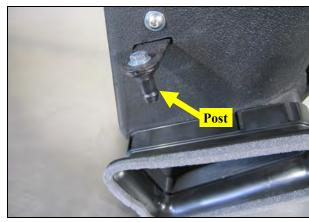
12. Install the Airbox Mounting Post onto the Bracket, as shown using the 6mm Hex Bolt and one Flat Wash-
