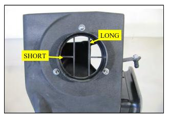
**13.** Install the Filter Adapter onto the Airbox using three sets of 1/4-20 Button Head Screws and Flat Washers. Note the positioning of the Adapter in the Airbox. When properly installed, the long air vanes are vertical and the short vanes are horizontal.
