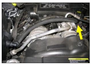
**8. 5.7 Hemi engines only**. Using the supplied straight <sup>3</sup>/<sub>4</sub>" hose, connect both ends to the nylon fitting and oil fill nipple as shown. Fasten both ends using the supplied nylon speed clamps. Adjust the nylon fitting downward to clear the factory intake tube assembly.
