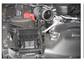
**2.** Loosen the hose clamp on the air box lid and remove the lid from the air box base.
