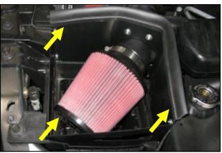
**9.** Install the Airaid Premium Filter on the end of the air filter adapter, and tighten the hose clamp. Install the supplied weather strip on the Cool Air Dam. (Note: start from one end and work your way around to insure proper alignment of weather strip.)
