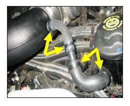
**17. <u>2003 Models Only:</u>** Use the plastic barbed fitting and ½" hose provided; connect factory vent hose to Airaid intake tube & secure the 1/2" hose with (2) #16 black speed clamps provided. Secure factory vent hose with (2) #22 black speed clamps provided.
