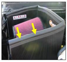
**19.** Install weather strip along the top rim of the Airaid Intake System. (Hint: start the install at the top corner of the cold air dam)
