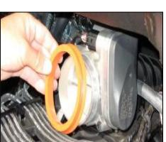
6. Remove the factory resonator and rubber seal from throttle body.
