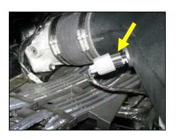
16. Re-connect air temperature sensor connector.
