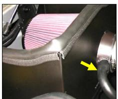
11. 2004-05 Models Only: Mount factory breather hose to the nipple on the Cool Air Dam and secure using the #24 black speed clamp provided.
