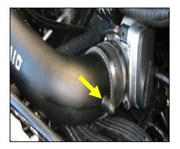
**18. <u>2004-05 Models Only:</u>** Slide the black rubber cap over the nipple near the throttle body end of the Airaid Tube.
