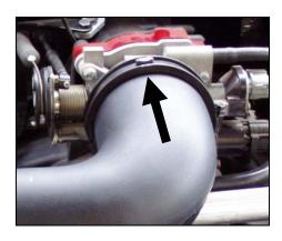
13. Factory coupler must be orientated with the clamp screw at the 12 o'clock position.
