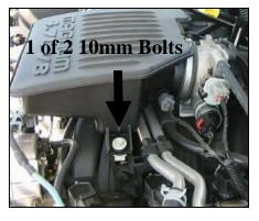
**5.** Loosen and remove the two 10mm bolts below the silencer box
