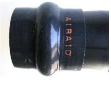
**10.** Install the urethane hump hose onto larger end of the Airaid Intake tube using the # 56 hose clamp provided.
