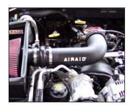
12. Slide the intake tube into the throttle body & align hump hose with Airaid Cool Air Dam. Slide the hump hose over end of the Airaid Cool Air Dam intake and secure using a #56 hose clamp.
