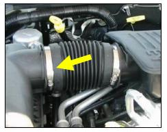
**1.** Disconnect negative battery cable and loosen the intake tube clamp.
