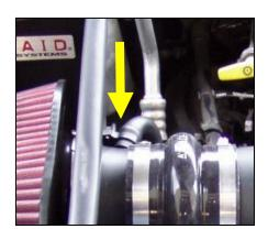
Reconnect the crankcase breather hose to the tube on the Airaid Cool Air Dam and secure with the black speed clamp provided. (Note for 2004: Replace breather hose with new 1/2" ID hose and speed clamps provided.)
