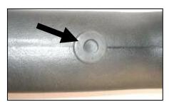
**15.** If your vehicle is not equipped with an air temperature sensor, insert the rubber grommet plug into the hole on the intake tube.
