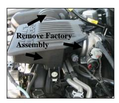
**6.** Loosen the hose clamp on the throttle body & remove the silencer box & accordion style tube from vehicle.
