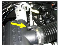
**2.** Disconnect the crankcase breather tube at the air box lid.
