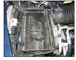
**3.** Unclip the factory air box lid and remove the lid and factory air filter from vehicle.
