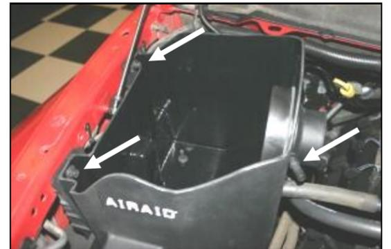
**9.** Install the CAD into the vehicle by aligning the grommets over the locating pins on the factory airbox mount. Reinstall the factory bolts in the fender that were removed in step #4. Next install the 1/4"NPT x 1/2" barbed fitting (#19) into the CAD. **2003 Models:** Install the 1/4"NPT plug (#22) in place of the barbed fitting.
