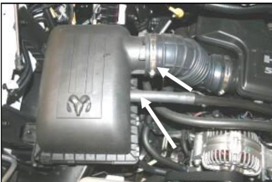
**1. Disconnect the negative battery cable!** Loosen the hose clamp on the flexible intake tube at the airbox lid. Disconnect the breather hose going into the factory airbox lid. Slide the flexible tube off of the lid and lift the airbox assembly straight up and out of the vehicle. **2003 Models:** Disconnect the breather hose from the back of the resonator.
