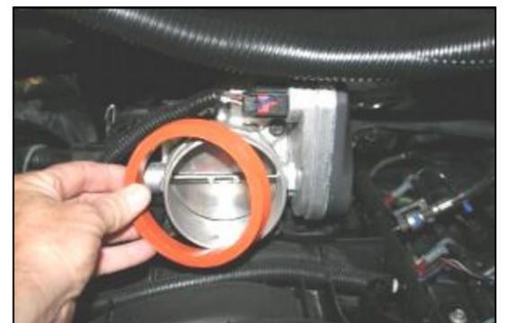
**3.** Remove the factory seal from the throttle body.
