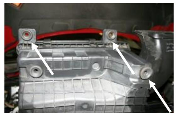
**6.** Remove and save three grommets from the bottom of the factory airbox. They will be reused in step #7.
