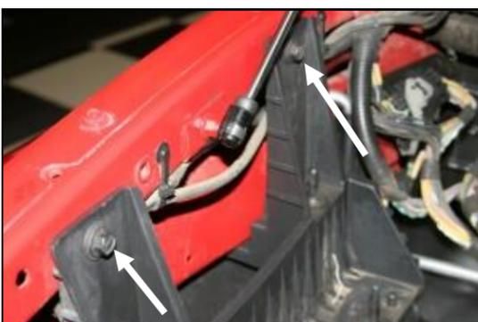
**4.** Using a 13mm socket, remove two bolts holding the airbox mounting bracket to the inner fender. These bolts will be reused in step #9.
