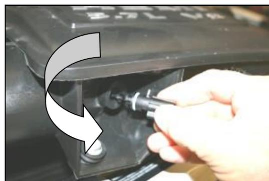
**5.** Gently twist the air temperature sensor counter-clockwise and remove it from the resonator. The sensor will be reinstalled in step #11.
