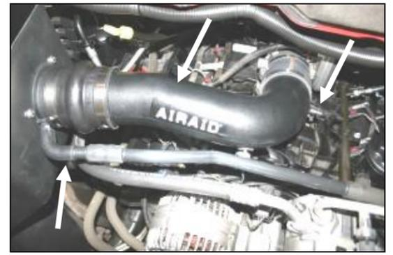
**12.** Install the Airaid intake tube into the hump hose first, and then into the reducing coupler. Adjust for fit, and then tighten all four hose clamps.
