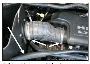
Reinstall the factory air intake tube and tighten the two hose clamps.
