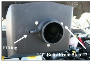
**7.** Install the 1/4" NPT x 1/2" barbed fitting (#8) into the filter adapter as shown. **2003 Models:** Install the 1/4"NPT plug (#10) in place of the barbed fitting.
