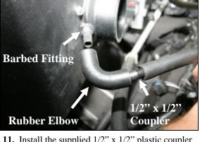
**11.** Install the supplied 1/2" x 1/2" plastic coupler (#11) into the 1/2" hose from step #10. Next connect the 1/2" rubber elbow (#8) between the 1/2" connector and the barbed fitting on the filter adapter.
