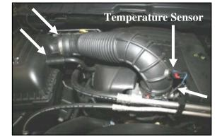
1. Disconnect the negative battery cable! Locate the temperature sensor on the air intake tube, slide the red tab, squeeze the black tab on the electrical connector, and then disconnect the temperature sensor from the air intake tube. Disconnect the crankcase breather tube from the air filter box. Loosen one hose clamp at each end of the air intake tube and remove it from the vehicle.
