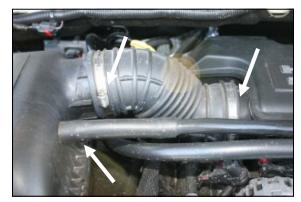
1. **Disconnect the negative battery cable!** Loosen the two hose clamps on the flexible intake tube, one at the airbox lid and one at the resonator. Slide the flexible tube off of the lid and the resonator and remove it from the vehicle. **2004-and later Models:** Disconnect the crank-
