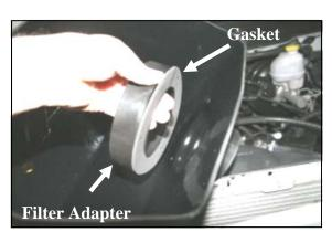
**6.** Install the adapter gasket (#12) and filter adapter (#3) into the **CAB** using three 1/4-20 x 5/8" bolts (#5) and flat washers (#6) as shown. *Refer to the line drawing above for reference*.
