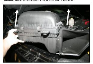
4. Rock the airbox back and forth as you are lifting it straight up to remove it from the vehicle. It is
