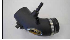
13. Install the provided step coupler onto the AIRAID<sup>®</sup> intake tube as shown.
