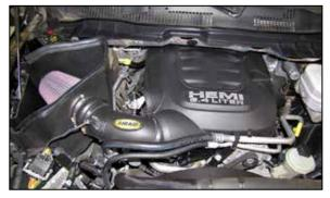
19. Double check your work! Make sure there is no foreign material in the intake path. Make sure all clamps, hoses, bolts, and screws are tight. Double check the hood clearance! **Reconnect the negative battery cable!**
