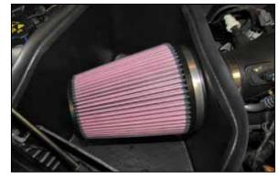
17. Install the air filter onto the filter adapter and secure with the provided hardware.
