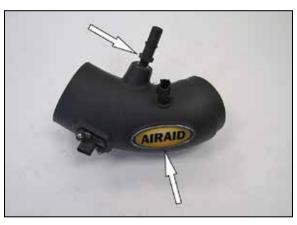
12. Install the provided quick connect vent fitting and AIRAID® decal onto the AIRAID® intake tube as shown. NOTE: Plastic NPT fittings are easy to cross thread. Install the vent fitting "hand" tight, then turn it two complete turns with a wrench.
