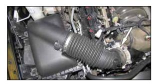
4. Loosen the hose clamp that secures the factory intake tube to the throttle body, release the four clips that secure the upper air filter housing and then remove the upper air filter housing and intake tube from the vehicle.
