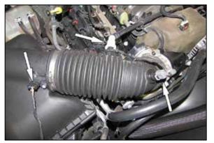
3. Disconnect the mass air sensor and inlet air temperature sensor electrical connections and disconnect the crank case vent quick connect fitting.
