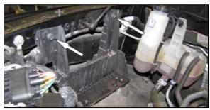
6. Remove the two upper filter housing bracket mounting bolts.
