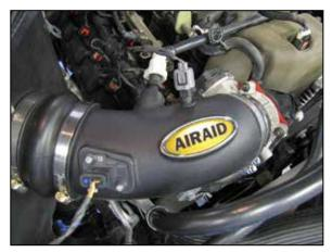
16. Connect the crank case vent to the fitting installed into the AIRAID<sup>®</sup> intake tube. Reconnect the mass air sensor and inlet air temperature sensor electrical connections.
