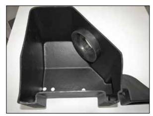
7. Install the filter adapter into the air box as shown and secure with the provided hardware.
