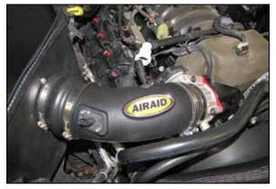
15. Install the AIRAID<sup>®</sup> intake tube into the hump coupler and onto the throttle body, adjust the tube and couplers for best fit and then secure with the provided hose clamps.
