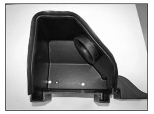
9. Install the provided wiper trim onto the AIRAID® filter housing as shown.
