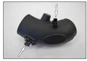
11. Remove the mass air sensor and inlet air temperature sensor from the factory air filter housing and install them into the AIRAID® intake tube with the provided hardware and grommet.
