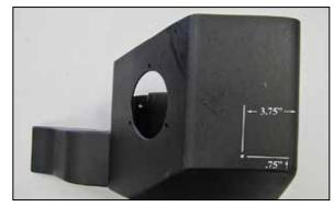
8a. On model that have the A/C lines and heater hose tube secured to the factory air filter housing, drill a  $\frac{1}{4}$ "id hole as shown to secure the heater hose tube.
