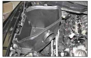
10. Install the AIRAID® filter housing onto the factory air filter housing mounting studs and secure with the hardware provided.
