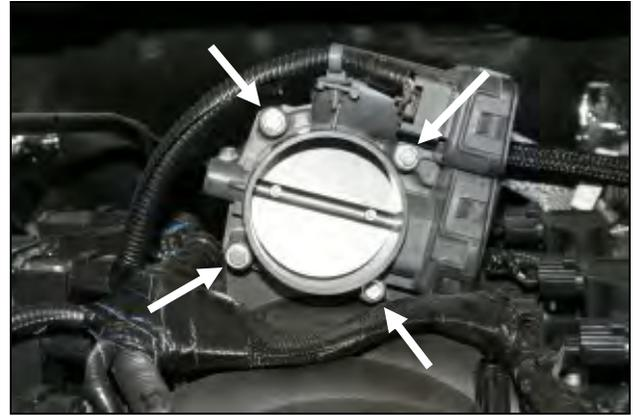
4. Install the provided bolts and washers thru the throttlebody and Airaid Spacer and tighten to the manufacturer's specifications.
