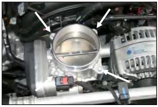
2. Remove the four bolts that secure the throttle body to the intake manifold. Without disconnecting the wiring harness, remove the throttle body from the intake manifold and set it
