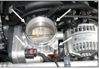
**5.** Reinstall the throttle body on top of the Airaid Spacer using the four bolts and the washers that were selected in step 3. Tighten the bolts evenly, in an X pattern, to the vehicle manufacturers specifications.
