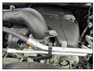
9. Reconnect the inlet air temperature sensor electrical connection.
