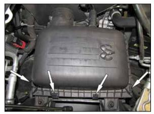
4. Release the clips retaining the upper air filter housing and remove the factory air filter.
