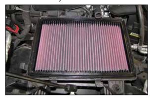
5. Install the provided AIRAID® air filter and then reinstall the factory upper housing and secure with the factory clips.
