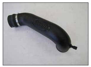
7. Remove the inlet air temperature sensor from the factory intake tube and then remove the O-ring from the sensor. Install the sensor into the AIRAID® intake tube using the provided grommet. Install the provided hump coupler (5-1074) onto the AIRAID® intake tube and secure with the provided hose clamp.
