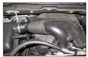
3. Loosen the hose clamps that secure the factory intake tube and then remove the intake tube from the vehicle. NOTE: AIRAID recommends that customers do not discard factory air intake.
