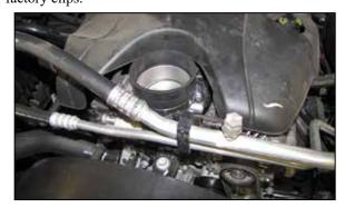
6. Install the provided coupler hose (08698) onto the throttle body and secure with the provided hose clamp.
