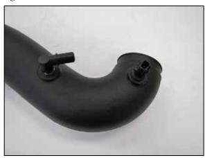
9. Install the Grommet supplied into the AIRAID® intake tube and then install the inlet air temperature sensor into the grommet. Install the provided vent fitting into the AIRAID intake tube as shown.
