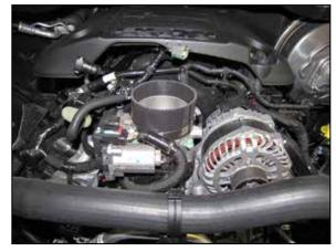
6. Install the coupling hose (KITCOUPLER09) onto the throttle body and secure with the provided hose clamp.
