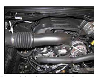
3. Loosen the hose clamps that secure the factory intake tube and then remove the intake tube from the vehicle.
