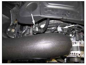
11. Reconnect the inlet air temperature sensor electrical connection and crank case vent line.
