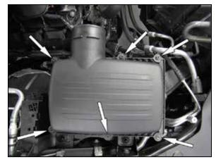
4. Loosen the six screws that secure the air filter housing lid and then remove the lid and factory air filter.
