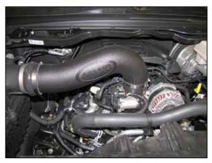
10. Install the AIRAID® intake tube into the coupler at the air filter housing and then into the coupler at the throttle body, adjust the tube for best fit and then secure with the provided hose clamps.
