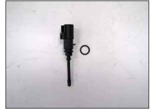
8. Remove the Inlet air temperature sensor from the factory intake tube and then remove O-ring from the sensor.
