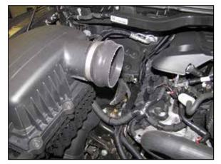
7. Install the provided hump coupler (KITHUMPHS35) onto the air filter housing and secure with the provided hose clamp.
