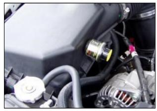
**2.** Remove the factory filter minder with grommet and retain for use with the Airaid Intake System.
