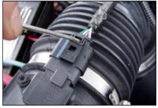
**1.Disconnect The Negative Battery Terminal!** Disconnect the electrical connector. Using the T-20 bit, loosen the two star head bolts and remove the electrical sensor. (Retain sensor for installation of Airaid Intake System)
