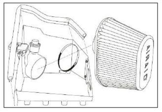
**10.** Mount Airaid Premium Filter to the filter adapter and tighten hose clamp. Next, press the weather strip onto the top of the Cool Air Dam (Hint: start at a corner and work toward the edges).
