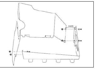
**5.** Assemble Airaid Quick Fit cool air dam panels using the (4) 6/32 bolts, washers and nuts provid-
