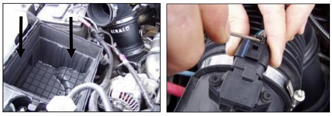
7. Fasten the factory sensor on top of the Airaid adapter using the (2) 8/32 screws and washers & a 3/32 Allen Wrench to tighten. In addition, mount the factory rubber grommet and filter minder onto the Airaid plastic adapter.
