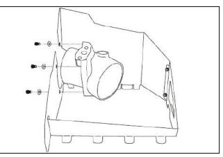
**6.** Assemble the air filter adapter to the cool air dam using the (3) <sup>1</sup>/<sub>4</sub>-20 bolts and washers provided.
