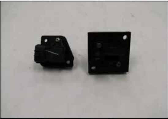
8. Remove the air sensors from the factory housing and install them into the K&N sensor adapters using the provided hardware.
