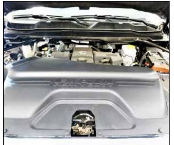
19. Reinstall the factory core support cover and secure with the factory retaining clips.
