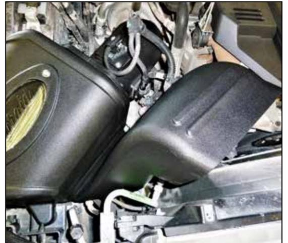
18. Install the AIRAID fresh air intake duct and then install the factory upper portion of the fresh air intake duct and secure with the factory hardware.
