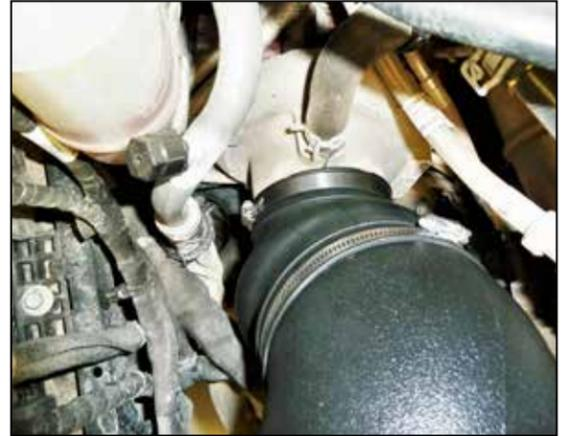
16. Secure the coupler to the turbo inlet with the provided hose clamp.
