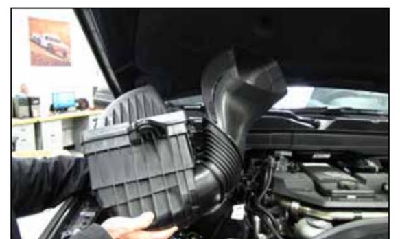
5. Remove the complete air filter housing from the vehicle as shown.
