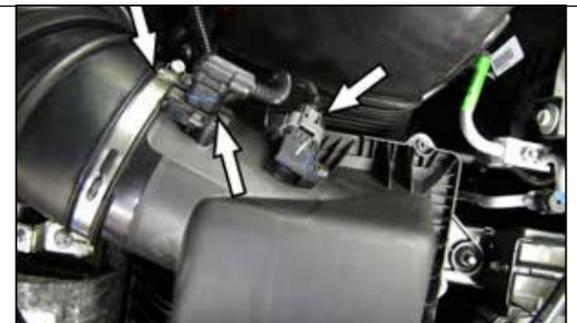
4. Loosen the hose clamp that secures the intake tube to the air filter housing and disconnect the electrical connections of the two air sensors.
