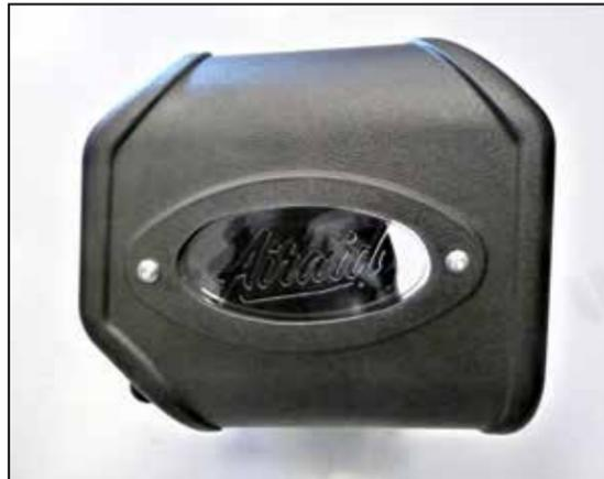
12. Install the AIRAID window into the air filter housing and secure with the provided hardware.
