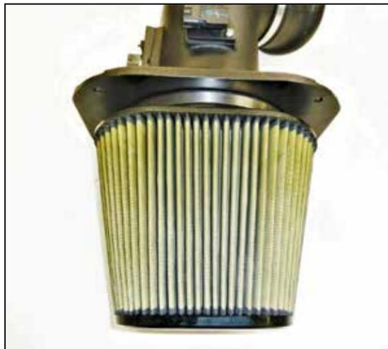
13. Install the AIRAID filter housing into the vehicle so the mounting pins protrude through the grommets.
