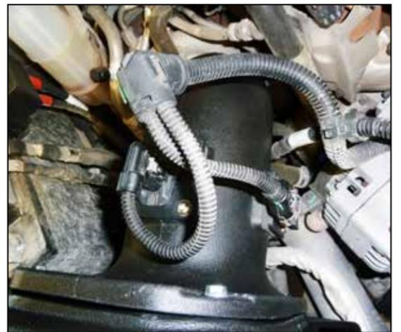
17. Reconnect the air sensor electrical connections.
