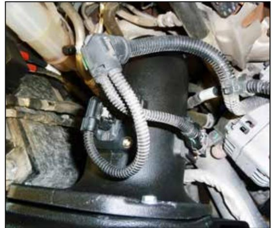
17. Reconnect the air sensor electrical connections.
