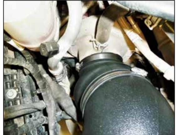
16. Secure the coupler to the turbo inlet with the provided hose clamp.
