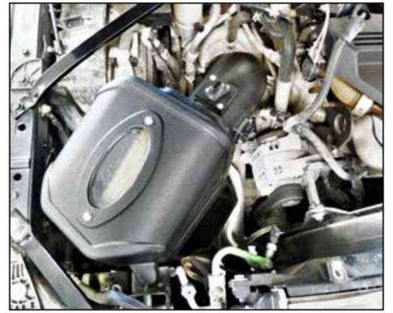
15. Install the intake system into the vehicle so the airbox rests on the mounting studs and connect the coupler to the turbo inlet.
