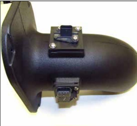
9. Install the two air sensor assemblies into the intake tube using the provided hardware. Be sure the top sensor is installed in the correct direction. The opening of the sensor should be towards the filter end of the tube.
