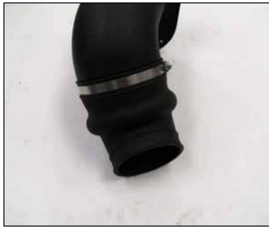
10. Install the flex coupler onto the intake tube and secure with the provided hose clamp. The coupler is keyed and can only be installed in one location.
