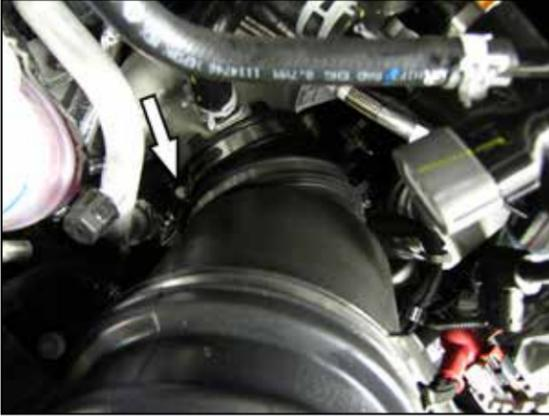
6. Loosen the hose clamp that secures the factory intake tube to the turbo inlet and then remove the tube from the vehicle.
