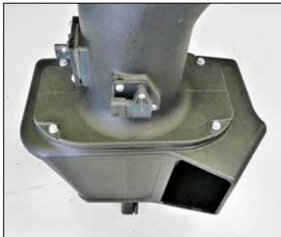
14. Install the tube assembly onto the filter housing. Secure the intake tube with the provided hardware.
