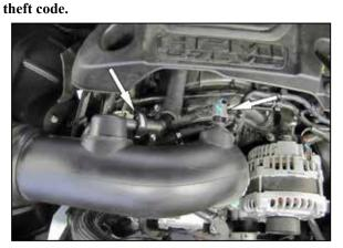
2. Disconnect the inlet air temperature sensor electrical connection and crank case vent quick disconnect fitting.
