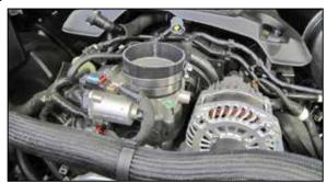
8. Install the provided coupler hose (KITCOUPLER09) onto the throttle body and secure with the provided hose clamp.
