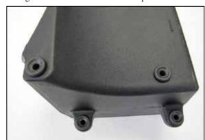
6. Remove the mounting grommets from the factory air filter housing and install them into the AIRAID® filter housing as shown.
