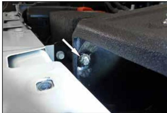
13. Install the air filter housing assembly into the vehicle so the mounting studs insert into the factory air filter housing mounting grommets, then align the housing with rubber mounted stud and secure with the provided hardware.
