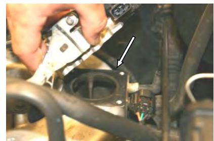
4. With the throttle body set aside, remove the gasケット and clean the surfaces of the manifold and throttle body.
