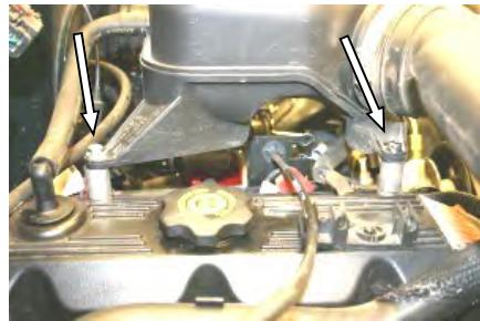
6. Install the two 1" aluminum spacers (#5) and provided 6mmx40mm bolts (#6) under the mounting tabs that hold the factory resonator to the top of the valve cover as shown.
