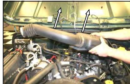
2. Remove the intake tube and resonator from the vehicle.
