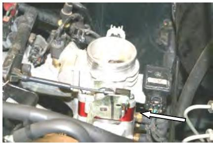
5. Install one gasket (#4) on the intake manifold, then the Airaid spacer (#1), with the other gasket (#4) on top of it. Next install the throttle body using the four provided 6mmx50mm bolts (#2) and washers (#3), and tighten to manufacturer's specifications.
