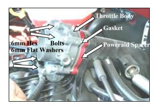
4. Install the Airaid Spacer (#1) with the bore extending into the intake manifold. Install the Gasket (#2) between the Airaid Spacer and the throttle body. Install four 6mm x 50mm hex bolts (#3) and 6mm flat washers (#4) through the throttle body, AiraidSpacer, Gasket, and into the intake manifold. Using a 10mm socket, tighten all four throttle body bolts evenly, to the manufacturer's specifications. Do Not Over Tighten The Bolts! Reference picture below for spacer orientation.
