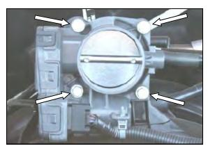
**3.** Using a 10mm socket, remove the four bolts that secure the throttle body to the intake manifold. Next, rotate the factory throttle body out of the way to allow access to the intake manifold. Make sure the factory blue gasket is seated in the groove on the intake manifold.
