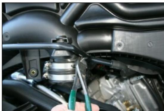
**5.** Carefully pull the intake towards you and rotate it so the bottom faces you, and cut the tie wrap that holds the breather tube, as shown.
