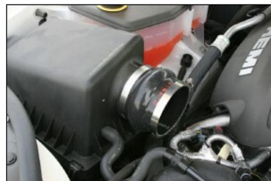
**9.** Reconnect the breather hose. Install the hump hose and two #60 hose clamps as shown. **Do not** tighten the clamps.
