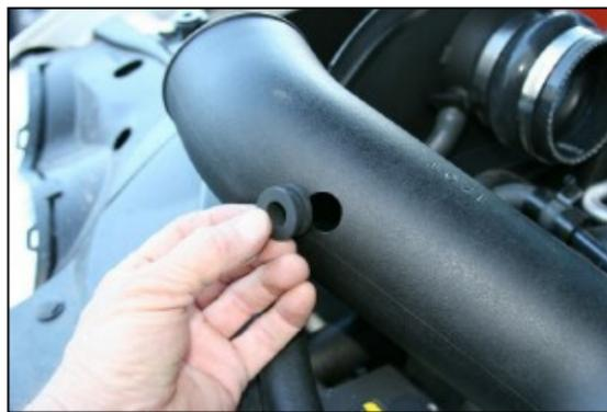
11. Install the supplied grommet into Airaid MIT as shown.
