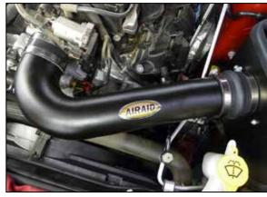
20. Install the AIRAID® intake tube into the silicone hump hose and then into the silicone hose at the throttle body, Secure the intake tube with the provided hose clamp.
