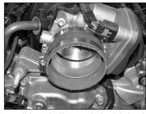
17. Install the provided hose onto the throttle body and secure with the provided hose clamp.
