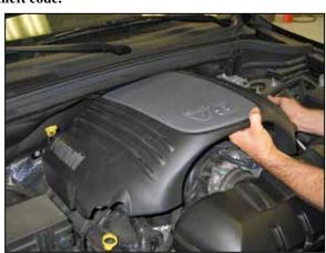
2. Lift up the engine cover to dislodge it from the mounting grommets and remove it from the vehicle.
