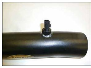
18. Release the locking tab and the remove the inlet air temperature sensor from the factory intake tube by twisting counter clockwise. Install the inlet air temperature sensor into the AIRAID® intake tube.
