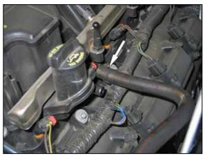
5. Disconnect the crankcase vent hose from the valve cover port.
