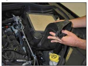
9. Lift up the lower airbox to dislodge it from the mounting grommets and then remove the lower airbox from the vehicle.
