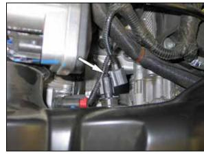
4. Disconnect the inlet air temperature air sensor electrical connection.
