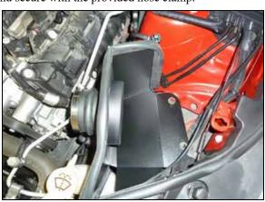
15. Set the heat shield into the vehicle so that the mounting grommets slide over the factory airbox mounting studs.
