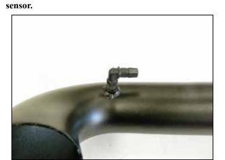
19. Install the 90° npt fitting into the AIRAID $^{\text{@}}$  intake tube as shown.
