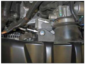
3. Remove the intake plenum mounting bolt shown and loosen the intake tube hose clamp.
