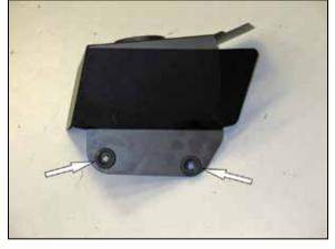
12. Install the two mounting grommets removed in the previous step into the heat shield as shown.
