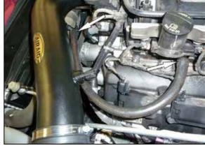
21. Install the crankcase vent hose onto the 90° vent fitting and then attach the open end to the valve cover
