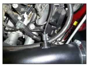
22. Connect the inlet air temperature sensor extension harness into the factory electrical connection and then connect the other end into the inlet air temperature sensor as shown.
