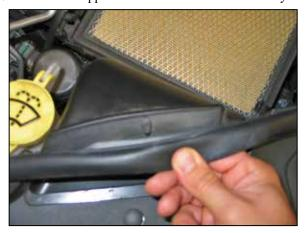
8. Unhook the sealing trim from the fresh air intake scoop.
