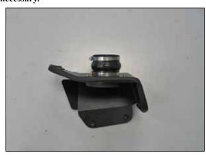
14. Install the provided hump hose onto the filter adapter and secure with the provided hose clamp.
