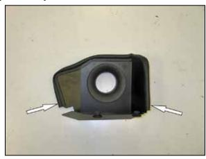
13. Install the provided edge trim onto the heat shield as shown.
