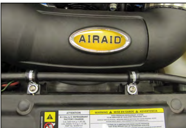
16. Secure the coolant line to the fan shroud using the two Adel Clamps, 6 mm Bolts, and 1/4" Flat Washers.
