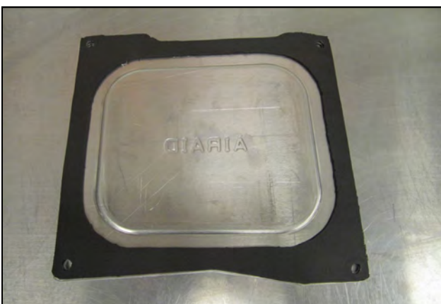
19. Place the Gasket onto the underside of the Air Box Lid and peel off the protective film. Mount the lid on the Air Box using four 1/4-20 x 1/2" Button Head Bolts, and 1/4" Flat washers.
