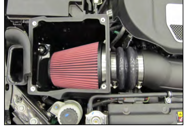
18. Install the Airaid Premium Filter onto the Filter Adapter.
