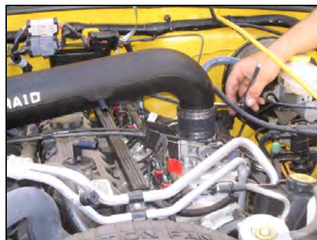
22. Install Airaid intake tube by connecting both ends into the urethane hump hose and reducer.
