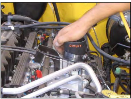
21. Install reducer coupler on throttle body with two #44 hose clamps. Leave hose clamps loose until final assembly.
