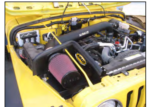
28. Install the weather strip on the edge of the Cool Air Dam assembly as shown above. Reconnect negative battery cable. Double-check your work to be certain that all nuts, bolts, and clamps are securely fastened.
