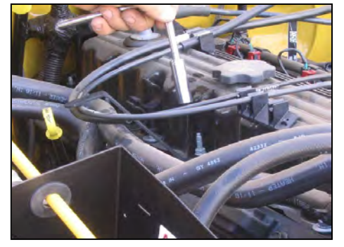
16. Remove one valve cover bolt on the passenger side nearest to the oil fill cap. Use this bolt to mount the supplied mounting bracket to the engine as shown above. Leave bolt loose until final assembly.
