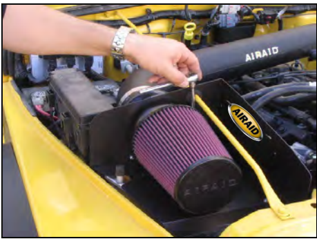
27. Install the Airaid Premium Filter on the Cool Air Dam assembly. Secure the filter using the supplied hose clamp.
