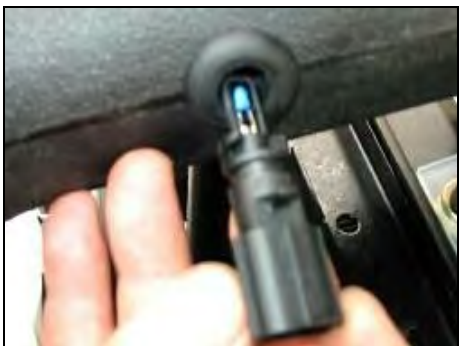
25. For 2005-06 Vehicles: Re-connect the air temp sensor on the backside of intake tube.
