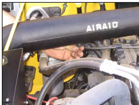
23. Mount the Airaid intake tube to the valve cover bracket using the supplied 1/4" bolt and washer as shown above.
