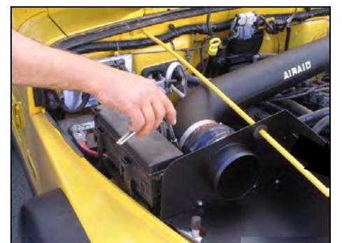
24. Make final adjustments to the intake tube for correct position. Tighten all four hose clamps and bracket.
