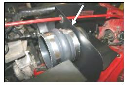
**16.** Install the hump hose (#5) onto the back side of the **CAD** tube using two #72 hose clamps (#17). Tighten <u>only</u> the hose clamp on the metal tube for now.
