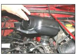
**6.** Remove the resonator from the vehicle.
