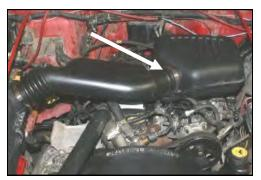
Disconnect the negative battery cable. Loosen the hose clamp that holds the factory intake tube to the resonator.
