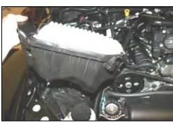
**5.** While rocking the factory air cleaner base back and forth, pull up, and remove it from the vehicle. There are no bolts holding it down, just grommets.
