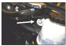
**8.** With a 10mm socket, remove and save the bolt that holds the radiator to the radiator support. It will be reused in step #10.
