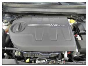
2. Lift up and remove the decorative engine cover to remove it from the engine.
