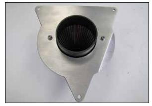
9. Install the air filter housing gasket and lid onto the radius adapter and secure with the provided hardware.
