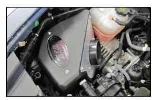
12. Install the AIRAID air filter housing assembly into the vehicle as shown so that it secures onto the factory housing mounting locations.
