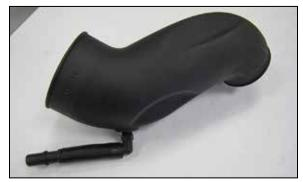
16. Install the assembled crank case hose assembly onto the AIRAID intake tube as shown.
