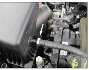
4. Disconnect the crank case quick connect fitting from the factory air filter housing. Pull up firmly on the air filter housing and remove it from the vehicle. **NOTE: AIRAID recommends that customers do not discard factory air intake.**
