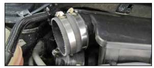
13. Install the provided coupler hose (08690) onto the intake plenum and secure with the provided hose clamps
