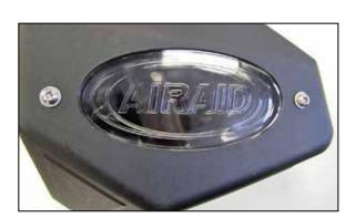
5. Install the AIRAID window into the AIRAID air filter housing using the provided hardware.
