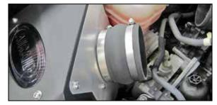
14. Install the provided coupler hose (08418) onto the filter adapter and secure with the provided hose clamp.
