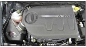
19. Reinstall the decorative engine cover. NOTE: It may be necessary to adjust the intake tube for clearance with the engine cover.
