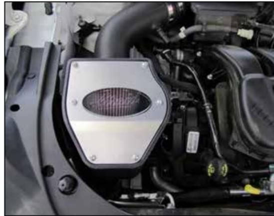
14. Install the lid onto the air filter housing and secure with the provided hardware.
