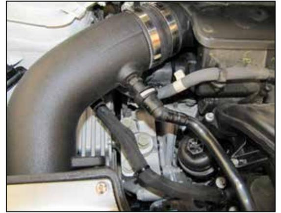
15. Connect the factory CCV hose to the quick connect fitting installed into the AIRAID intake tube.
