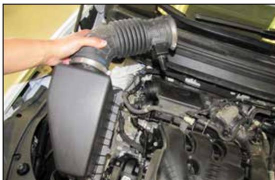
4. Loosen the hose clamp that secures the intake tube to the intake plenum. Disconnect the intake tube and then remove the complete intake system.
