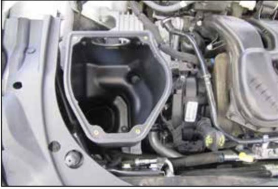
7. Install the AIRAID air filter housing into the vehicle so the mounting grommets and studs engage.
