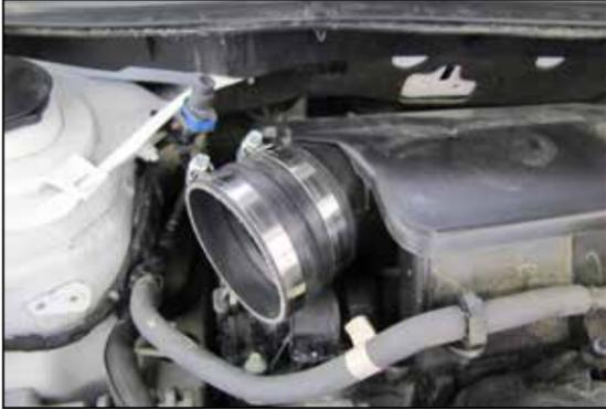
8. Install the provided coupler onto the intake plenum and secure with the provided hose clamp.
