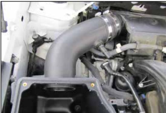
10. Install the intake tube into the coupler and AIRAID air filter housing and then secure with the provided hose clamp and hardware.
