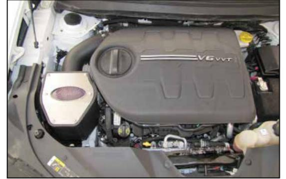
16. Reinstall the engine cover. Reconnect the negative battery cable.
