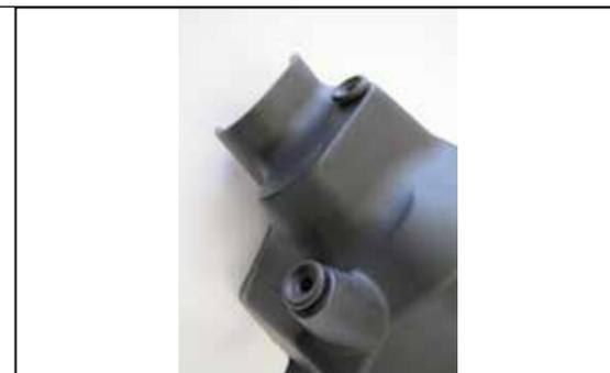
5. Remove the two factory mounting grommets from the factory air filter housing and install them into the AIRAID air filter housing as shown.
